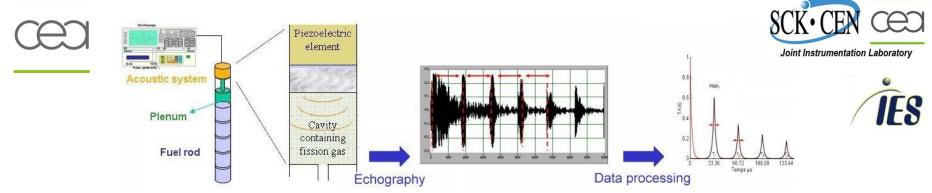
Online measurement of the molar mass of the gas inside the fuel rod ( $\rightarrow$  fraction of released fission gas)
