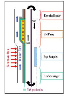
Diagram of the CALIPSO loop
